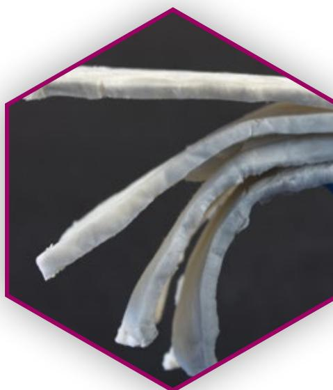
Empa researchers combined cellulose-based aerogels with silver nanowires. The flexible composite blocks high-frequency electromagnetic radiation, which is traditionally achieved by using inflexible metal sheets or metallized foils.
