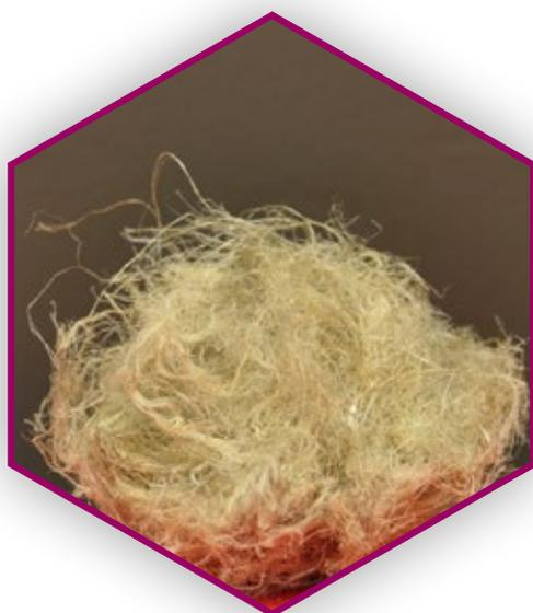
BFTi produces compostable fibre products out of agricultural waste from hemp and flax processing. Using biogenic waste from the production of fast-growing crops instead of using wood or fossil resources is environmentally and economically more sustainable.
