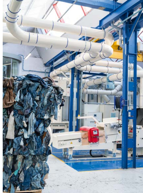
Technical center at ANDRITZ Laroche, France: Tearing lines to process any kind of textile and nonwoven waste
