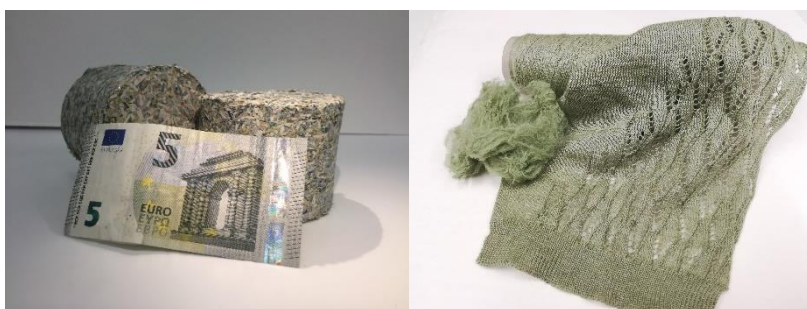
Figure1: Illustration of the initial banknotes (left) and the produced textile (right).
