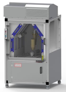
Lab scale line for nanofiber centrifugal electrospinning
