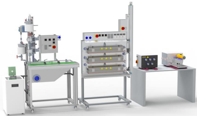
Lab scale line for wet spinning
