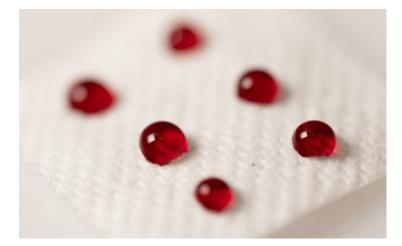
A picture of a cellulosic nonwoven which is coated with a bio-based substance, displaying its water-repellent properties. The water droplets on the surface are colored for enhanced visibility. This cellulosic nonwoven was produced from bio-based and biodegradable materials, ensuring it returns to nature with minimal environmental impact.
