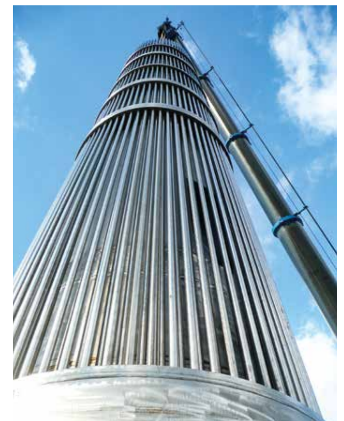
Short-path evaporator with integrated condenser © GIG Karasek
