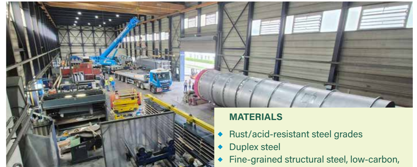
Cylinders with a diameter of up to 4,300 mm can be produced in Gloggnitz. © GIG Karasek
