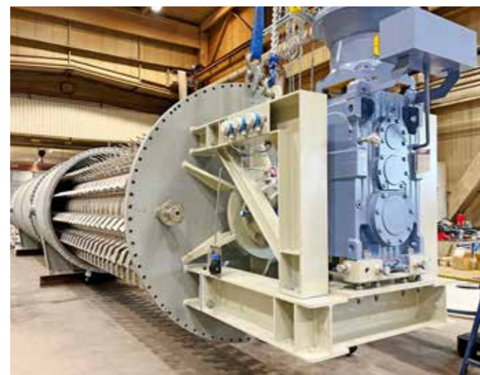
Horizontal thin-film dryer © GIG Karasek
