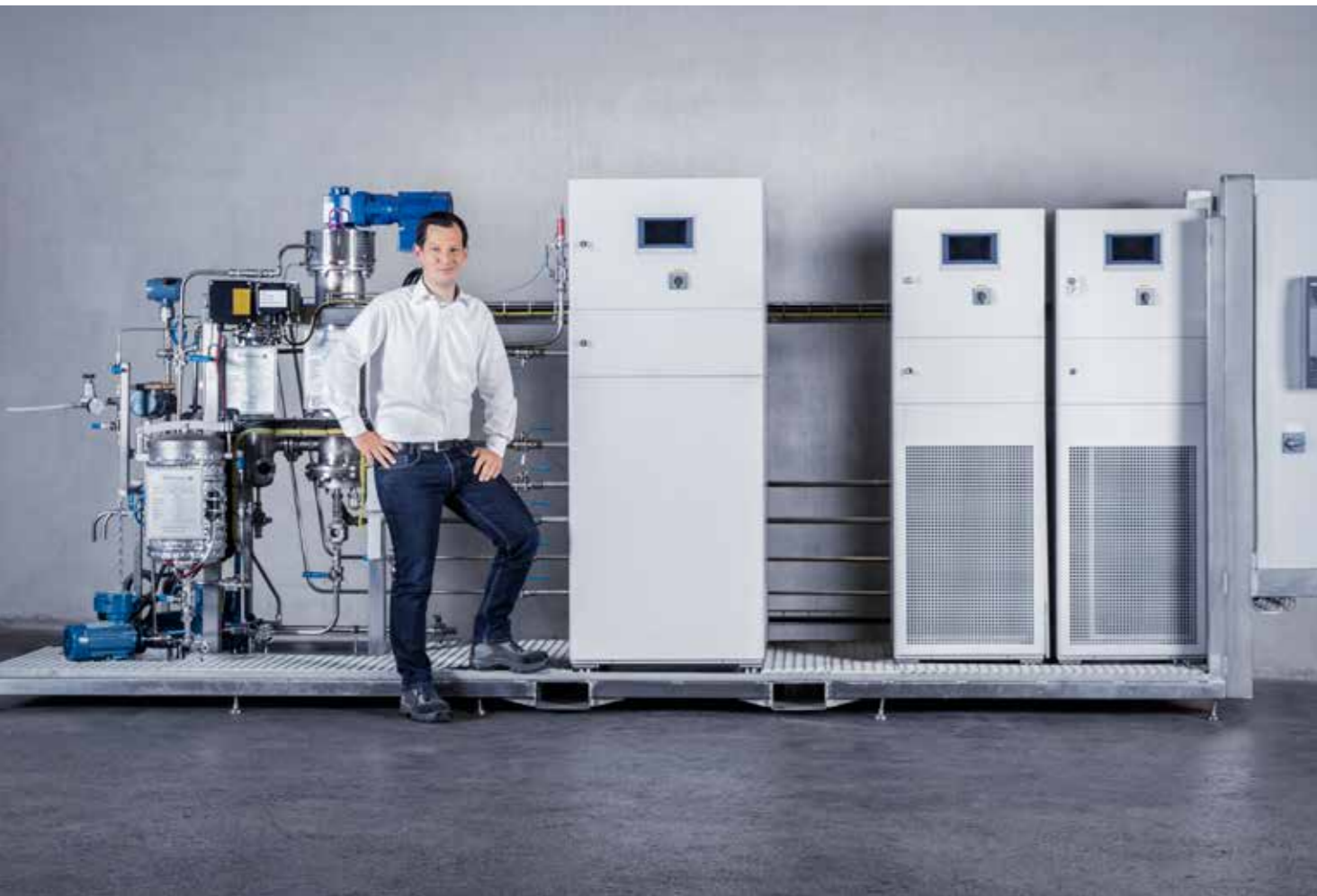
Short-path evaporator mini-plant for distillative purification and recovery of valuable materials © GIG Karasek
